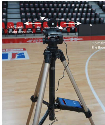
Vertical illuminance (EV) measurement
