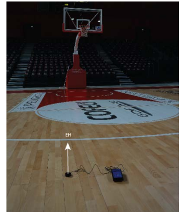
Horizontal illuminance (EH) measurement
